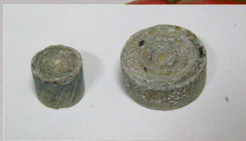
Fig. 1. Soil-improvers granules obtained on base of biomass ash and green lye
